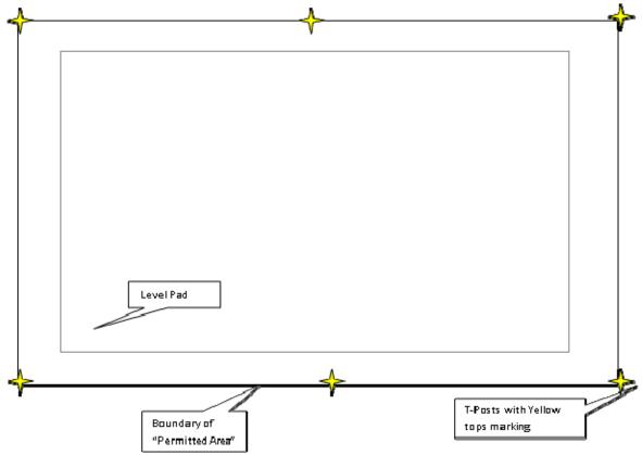
The following diagram is an example of the total useable area and the location of the T-post placement. T-posts will be placed after project approval but before construction on all well pads and compressor sites.
